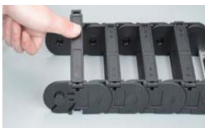
旋转横杆到另一侧 Swiveling crossbar to another side
