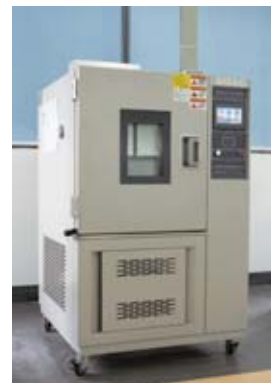
高低温交变试验箱 High and low temperature alternating test chamber
