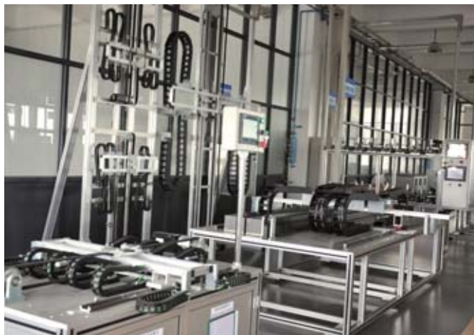
DURAMOV® 电缆拖链测试中心 DURAMOV® Plastic cable carrier test center
