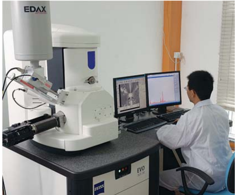
能谱仪 (EDS) Energy dispersive spectrometry (EDS)
